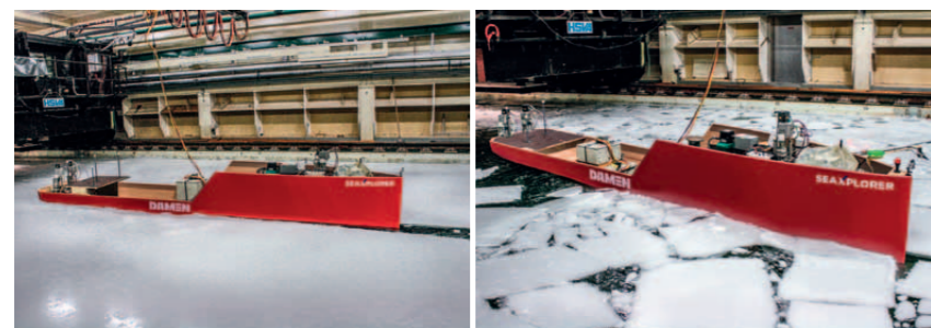
Shipping grade tank test: “SeaXplorer” had to demonstrate her ice-breaker qualities using both her stern and bow at the well-known Hamburg Ship Model Basin (HSVA).
